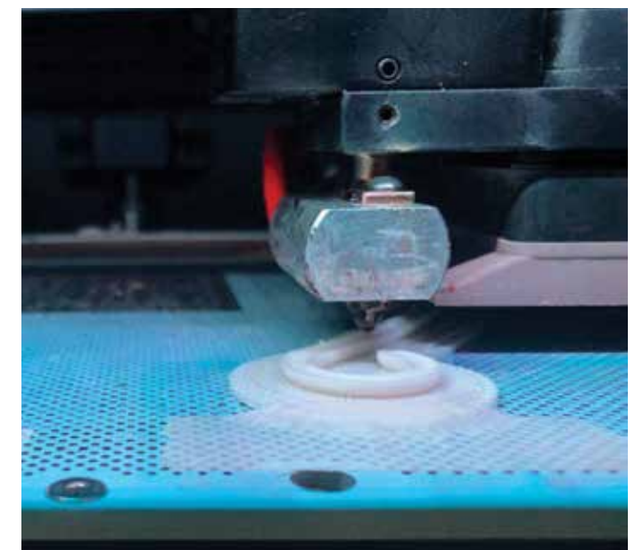
A closeup view of protective visors on a 3D printer. Photo Credit: Jenny Sabin Studio.
