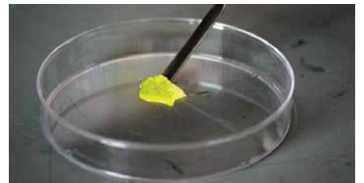
The researchers developed a collagen gel that incorporates riboflavin, a photoactive vitamin B derivative. When a light is shined on it, the riboflavin is activated and the thick gel stiffens into a solid. Video: cornell.edu/video/two-step-method-patches-herniated-discs .
